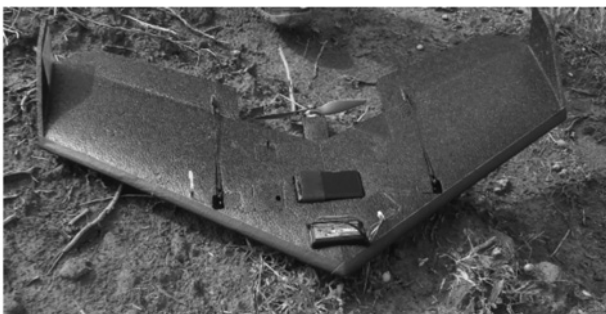
Figure 3. Swinglet with modified Canon IXUS 220HS.
