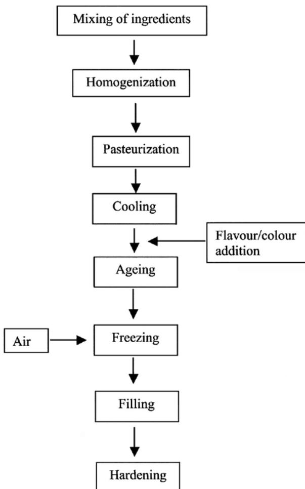
Figure 1. Flow chart for the production of red palm-based ice-cream.
