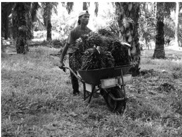
Figure 4. Collecting bunches using battery-powered wheelbarrow (BPW) along the harvesting path.
