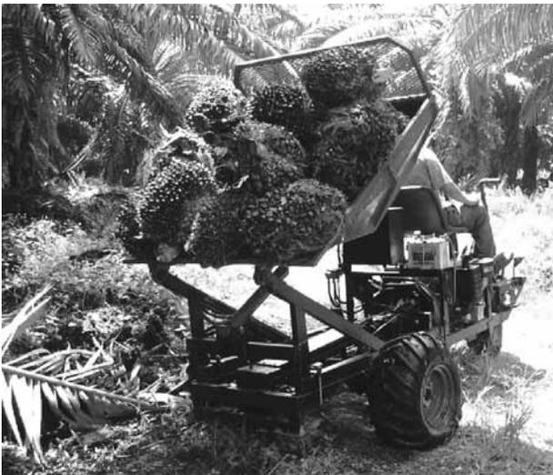
Figure 6. High pivot discharge mechanism of the three-wheeler power cart.
