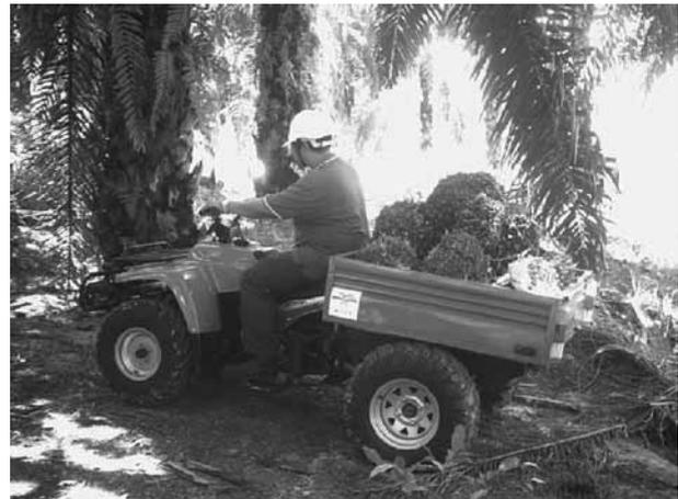
Figure 2. Compact transporter collecting fruit bunches along a narrow path.
