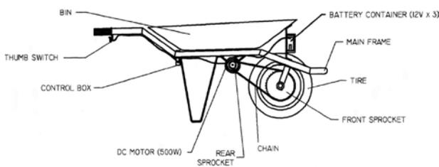
Figure 3. Configuration of the battery-powered wheelbarrow (BPW).
