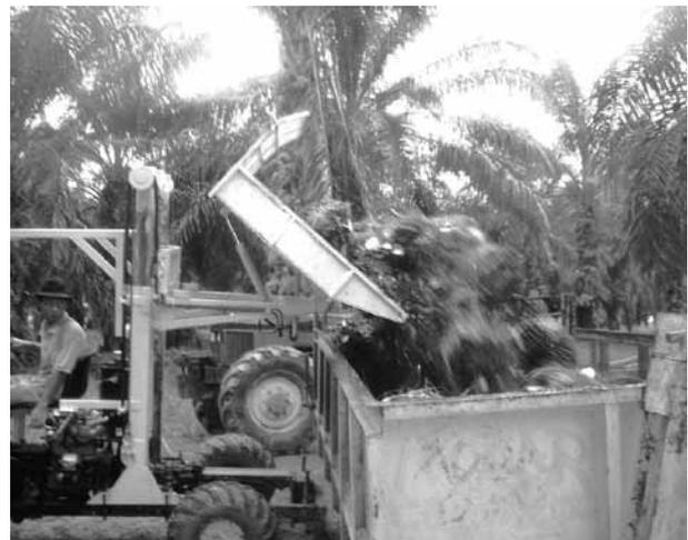
Figure 5b. Direct unloading of fruit bunches into a bucket using the 800 HP.
