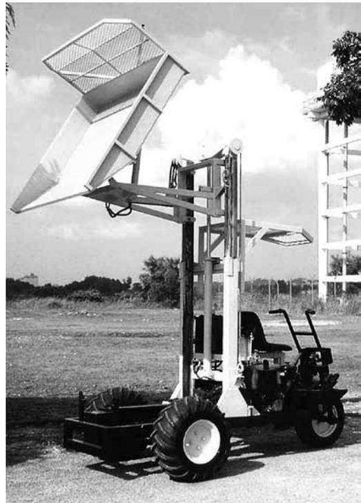
Figure 5a. High discharge point with a fork-lift concept of the 800 HP.
