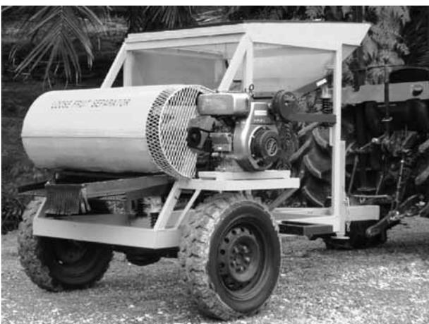
Figure 9. The air-assisted loose fruit separating machine.
