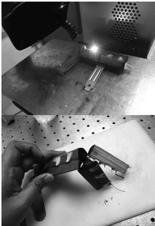
Figure 12. The laser cutting experiment on palm fronds.
