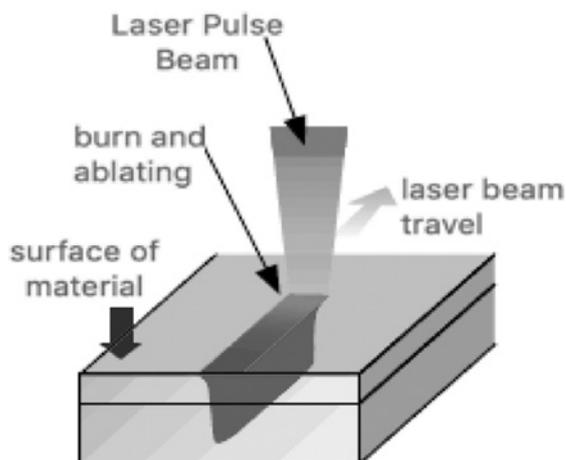
Figure 14. The movement of laser cutting on oil palm frond surface.
