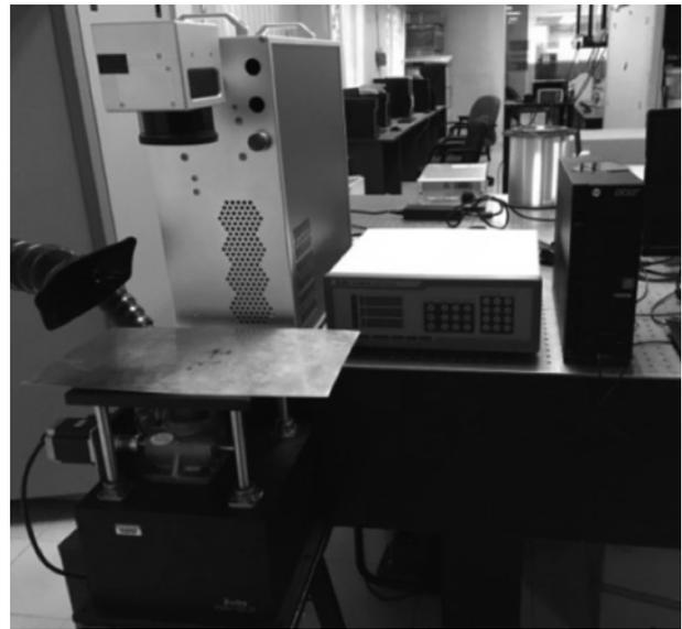
Figure 10. The pulse fibre laser system with an average power of 50W.
