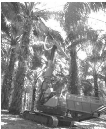
Figure 2. Mechanical harvesting machine.
