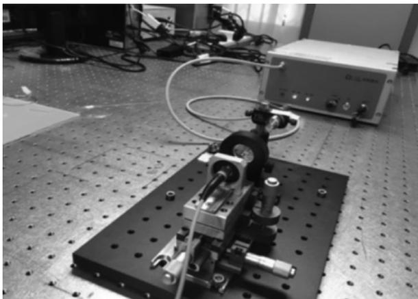
Figure 5. A wideband supercontinuum laser system.
