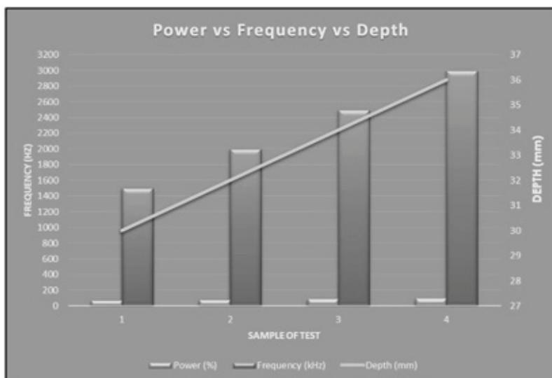
Figure 13. The comparison of different frequency with average power and speed reflect cutting depth.
