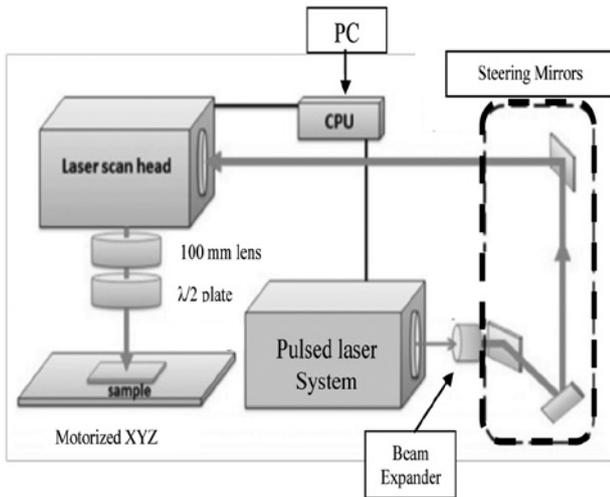
Figure 7. The diagram of installation of the laser system equipment.
