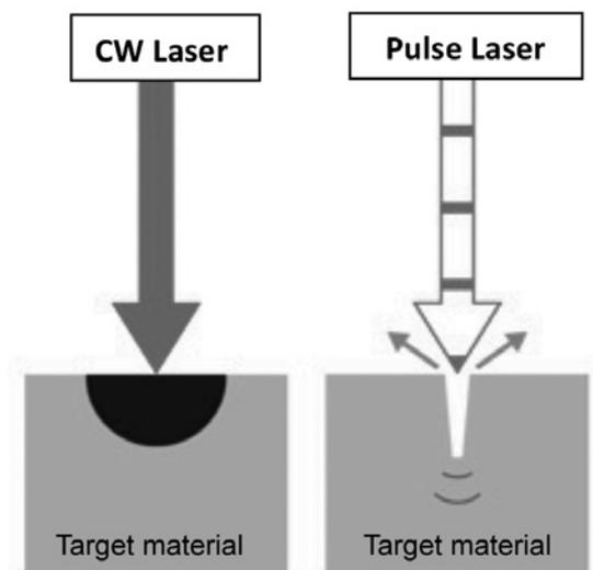
Figure 9. The difference between CW laser and Pulse Laser cutting.
