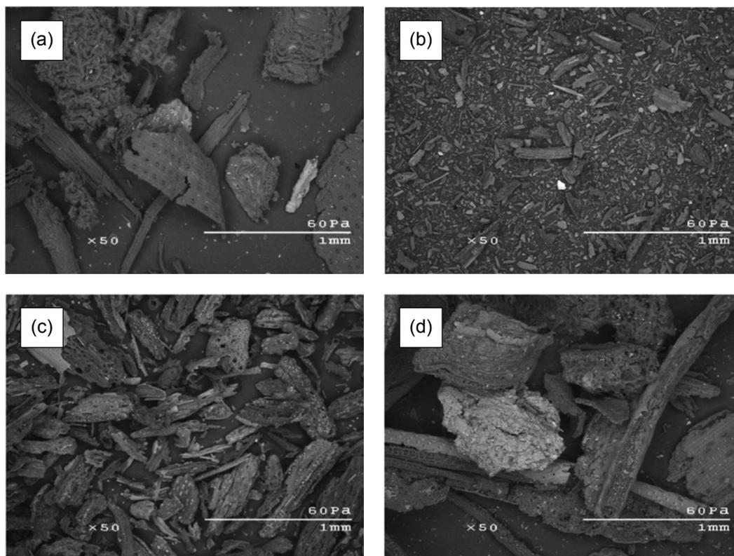
Figure 2. Scanning electron microscopy (SEM) images of (a) switchgrass feedstock, (b) slow pyrolysis biochar, (c) gasification and (d) fast pyrolysis biochar (pictures from Brewer et al., 2009) showed difference in porous structure that effects the quality of the pyrolysed products.
