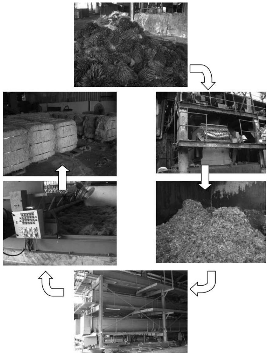
*Figure 2. Stages in empty fruit bunches (EFB) fibre production.*
