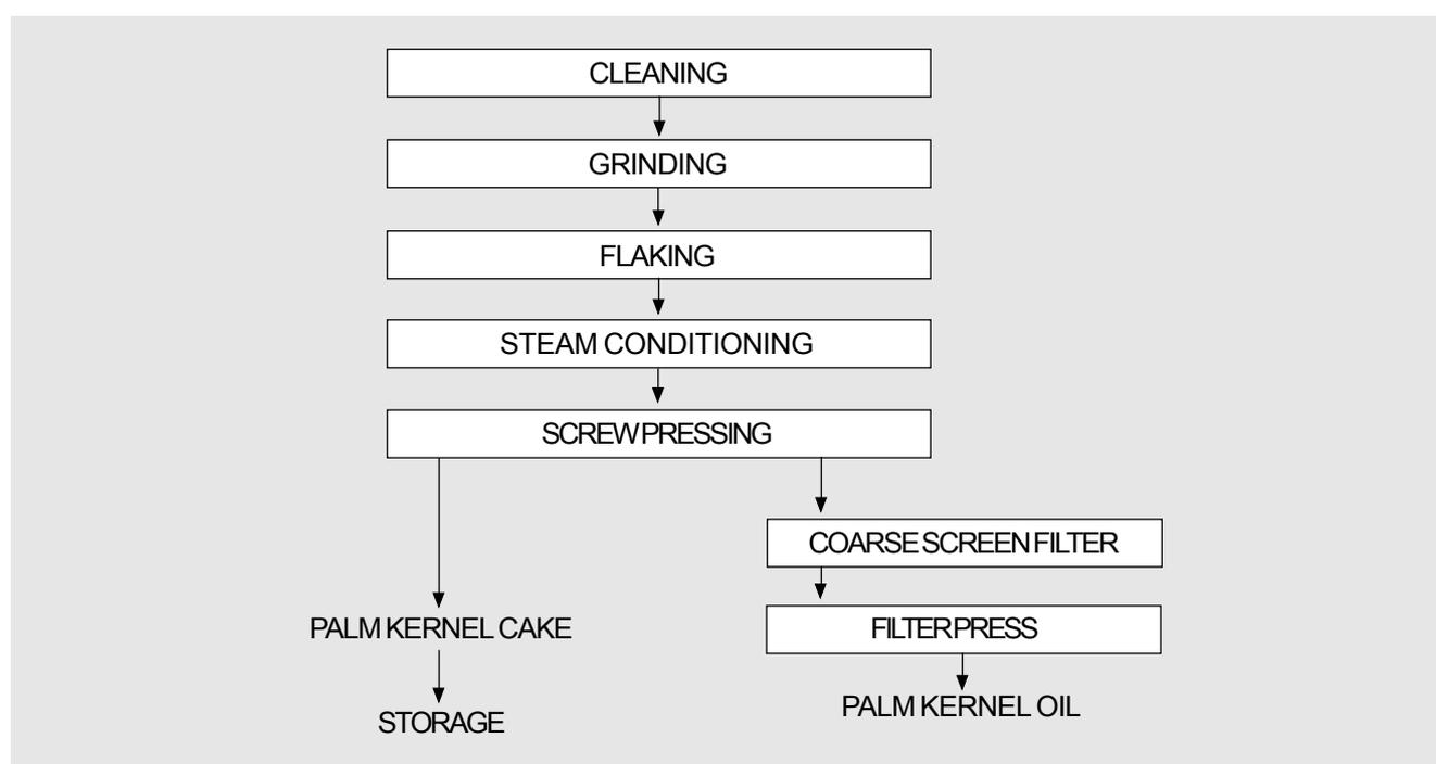
Figure 1. Mechanical extraction of palm kernel oil.
