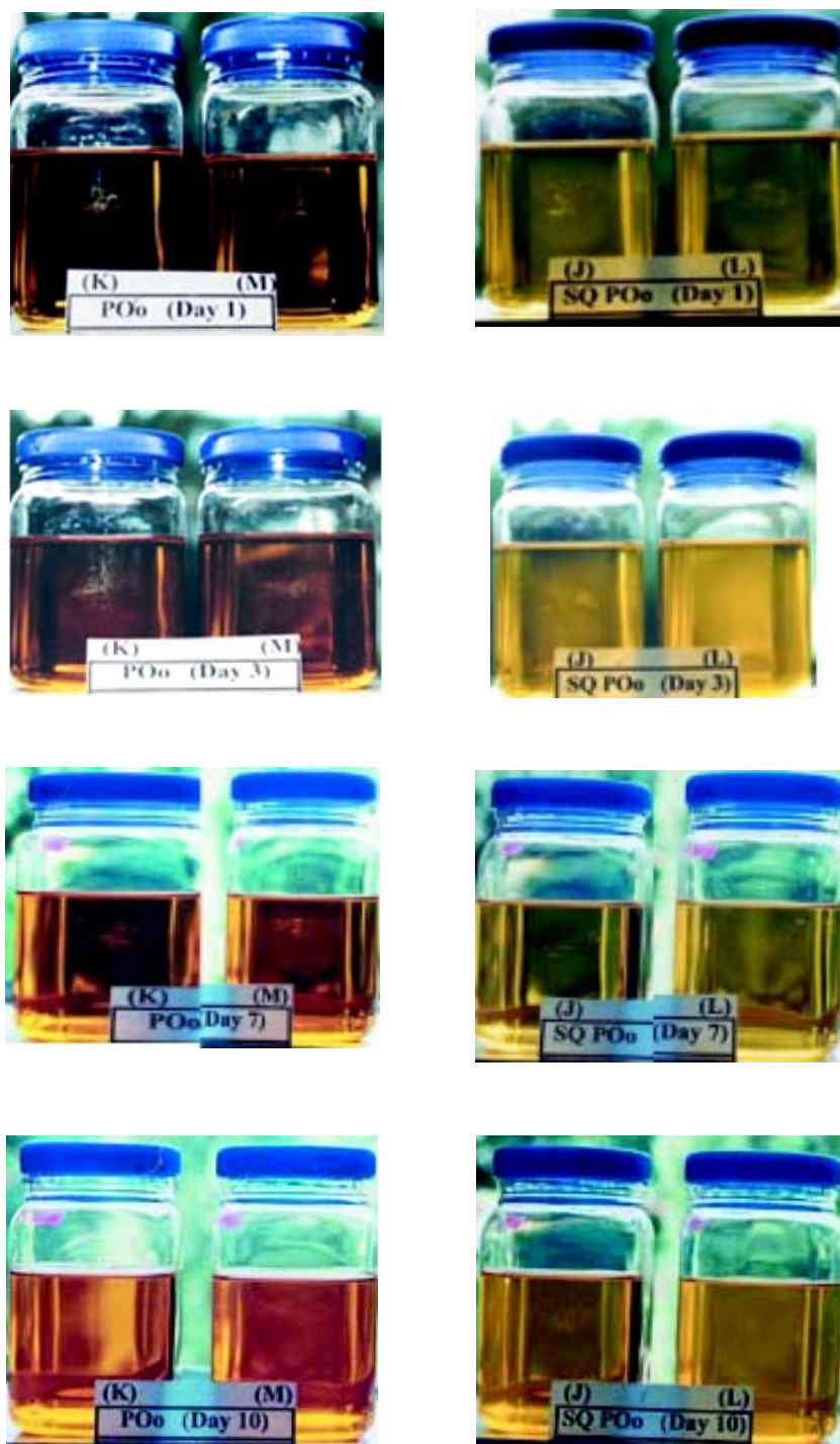
Figure 5. Changes in colour of special quality palm olein (SQ POo) and standard palm olein (POo) during frying.
