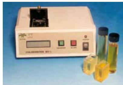
*Figure 4. Automatic colorimeter for palm oil.*
