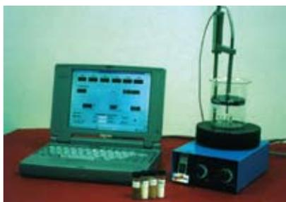
*Figure 3. Slip Melting Point Meter.*
