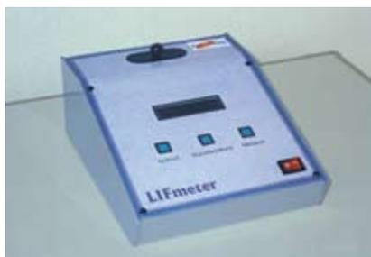
Figure 1. Laser Induced Fluorescence Spectrofluorimeter (LIFmeter).
