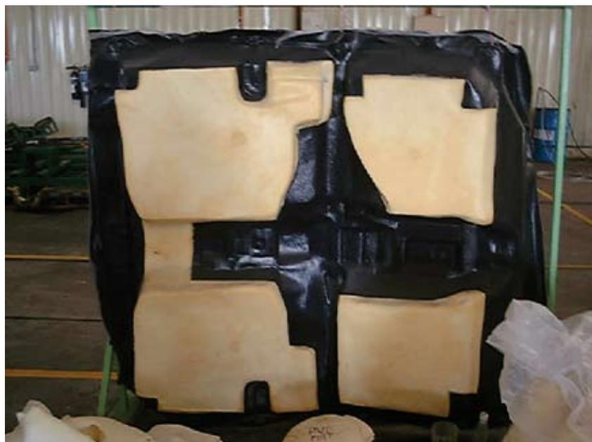
Figure 8. Palm oil-based polyurethane carpet underlay.
