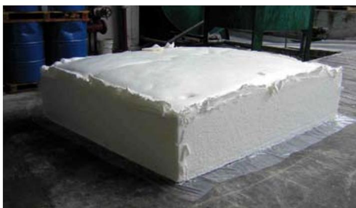
Figure 6. Palm oil-based flexible polyurethane slabstock.
