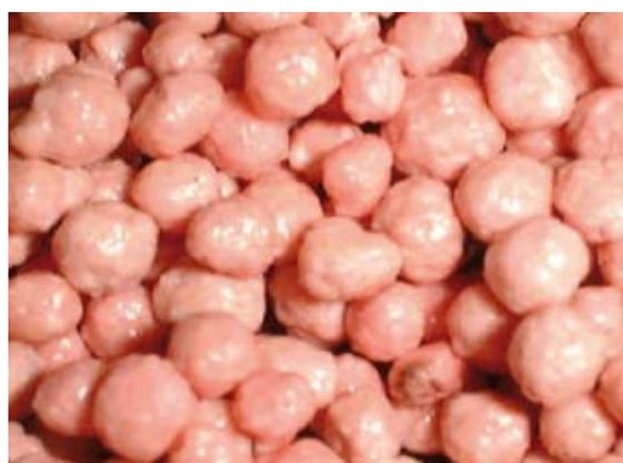
Figure 7. Palm oil-based polyurethane coated fertilizer.
