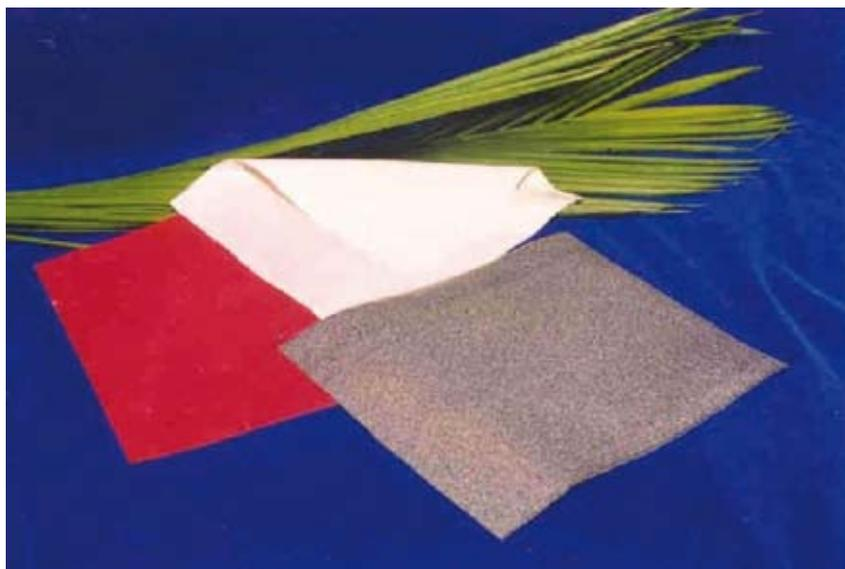
Figure 5. Palm-based polyurethane sheets.
