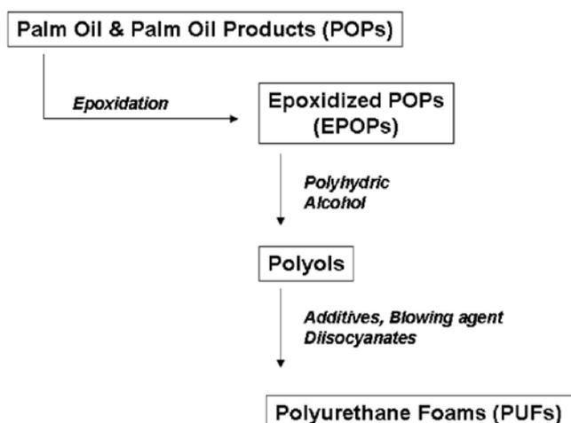
Figure 1. Process route for production of polyurethane foams.
