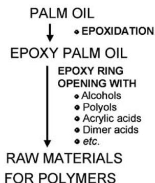
Figure 23. Raw material for polymers from palm oil.
