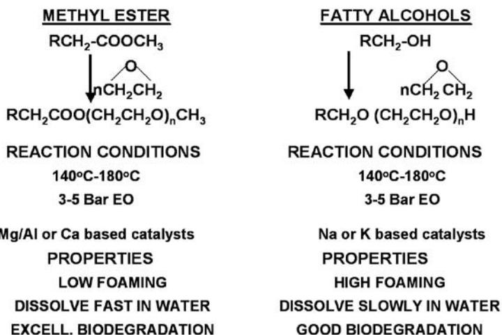
Figure 24. Nonionic surfactants through ethoxylation.
