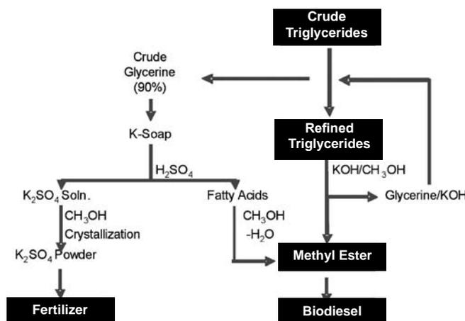
Figure 12. Environment friendly methyl ester process for biodiesel.
