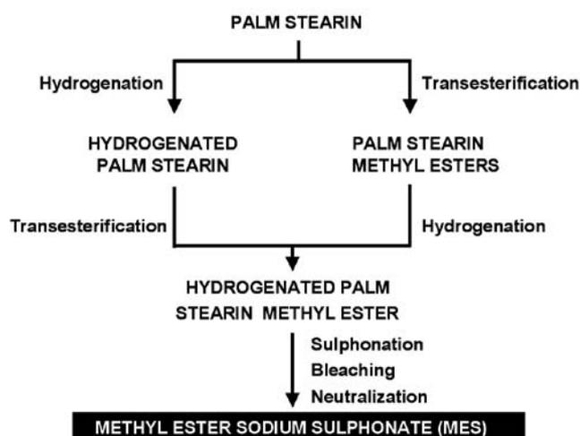
Figure 22. Methyl ester sulphonate from palm stearin.
