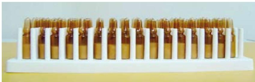
Figure 3. A series of Palm-based SRMs in the 5 ml dark amber glass ampoules.
