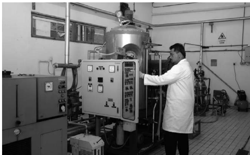
Figure 9. Multi-purpose vessel for refining and interesterification.
