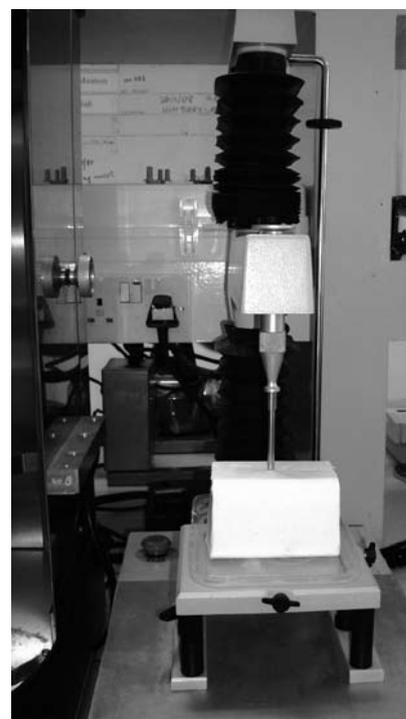
Figure 4. TA-XT2 model texture analyser (Stable Micro System USA).
