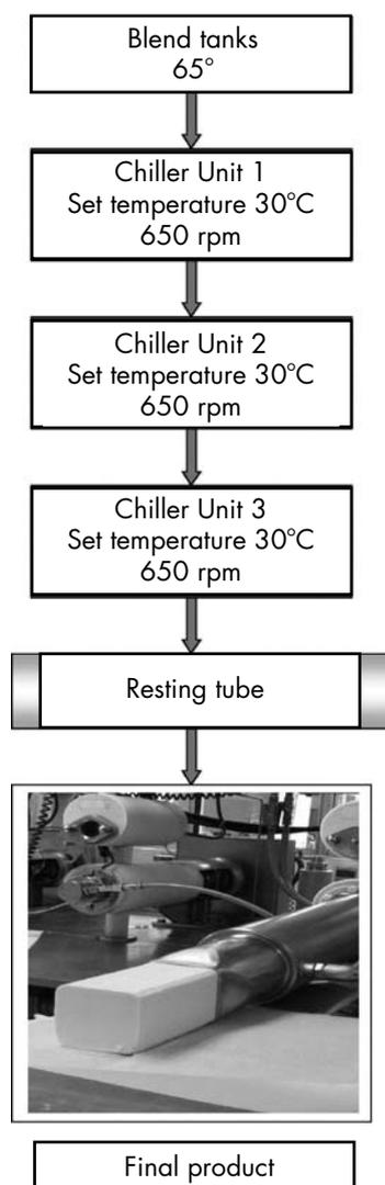
Figure 3. Flow chart of the processing conditions for the production of palm-based roll-in margarine.
