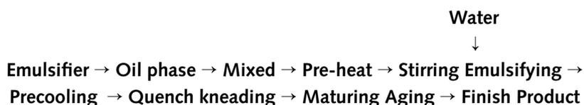
Figure 4. Process technology for palm-based special oil.
