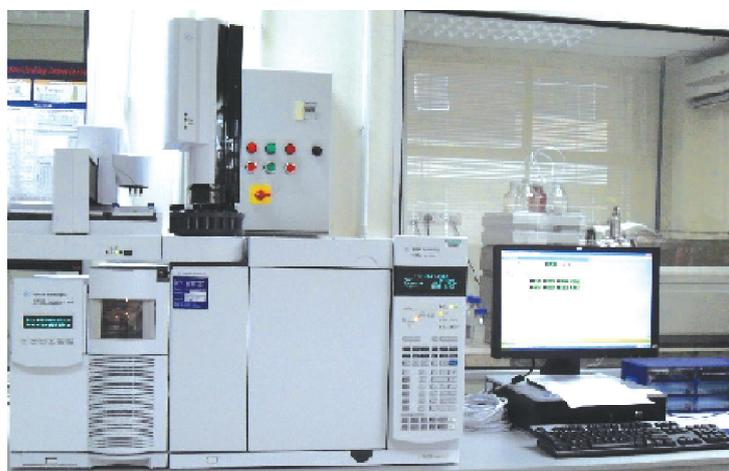
*Figure 2.* Gas Chromatography-Mass Selective Detector (GC-MSD) in Food Safety Laboratory, Malaysian Palm Oil Board.
