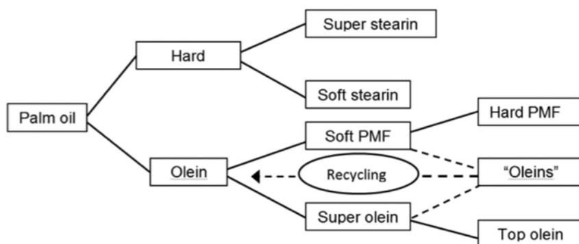
Figure 1. Dry fractionation of palm oil and its products from single-, double- and triple-stage dry fractionation.
