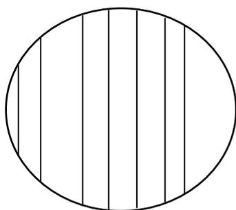
Figure 1. Live sawing.
