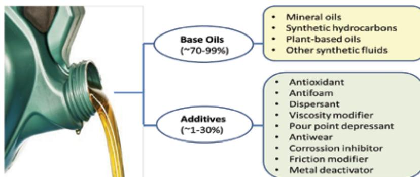
Figure 1. General composition of a lubricant formulation.
