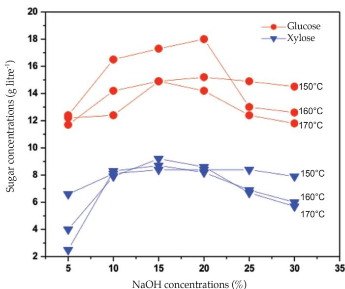
Figure 3. Effect of digestion temperatures of (a) 150°C, (b) 160°C and (c) 170°C on the extraction of fermentable sugars with various sodium hydroxide (NaOH) concentrations (digestion period of 200 s).
