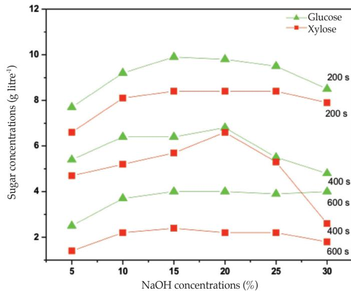
Figure 2. Effect of retention time of (a) 200 s, (b) 400 s and (c) 600 s on the extraction of fermentable sugars with various sodium hydroxide (NaOH) concentrations (digestion temperature of  $150^{\circ}\text{C}$ ).
