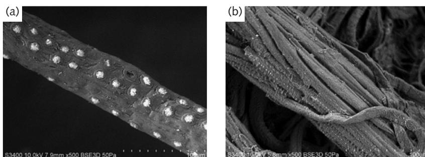
Figure 4. Scanning electron microscopy (SEM) micrographs (500X) of (a) untreated empty fruit bunches (EFB) and (b) EFB treated with 20% NaOH for 200 s (at digestion temperature of 160°C).
