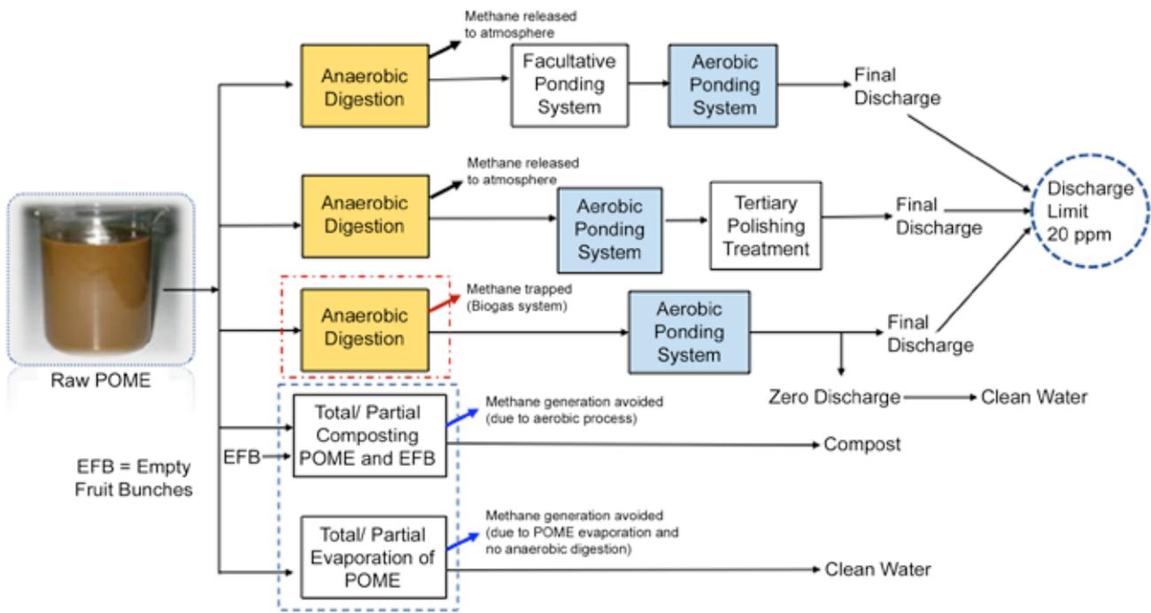
Figure 1. Different approaches in palm oil mill effluent (POME) treatment.
