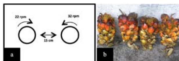
Figure 2. (a) An illustration of a gap and rotation of rollers in the bunch crusher and (b) spikelet of the oil palm bunch after crushed.
