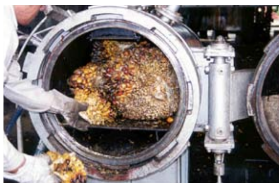
Figure 7. Crushed bunches preheating in autoclave.
