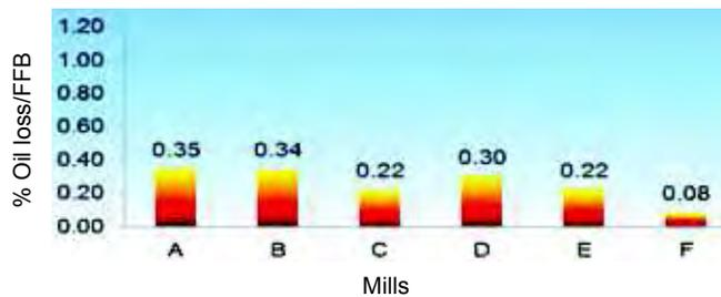
Figure 9. Percentage of oil loss to fresh fruit bunches (FFB) from steriliser condensate.
