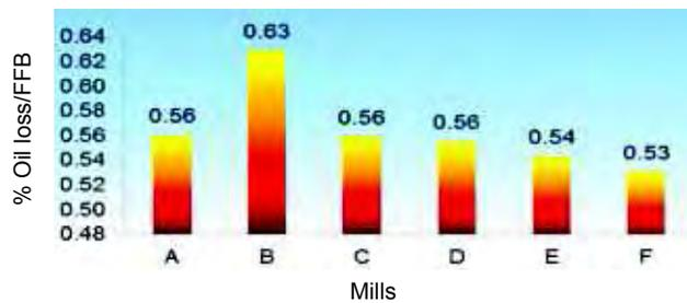
Figure 8. Percentage of oil loss to fresh fruit bunches (FFB) from press cake fibre.
