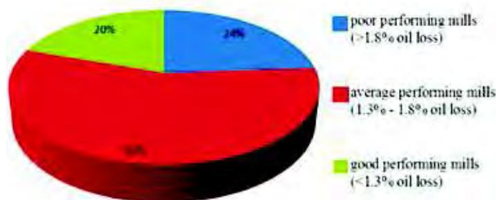
Figure 2. Survey on oil losses of oil palm mills.
