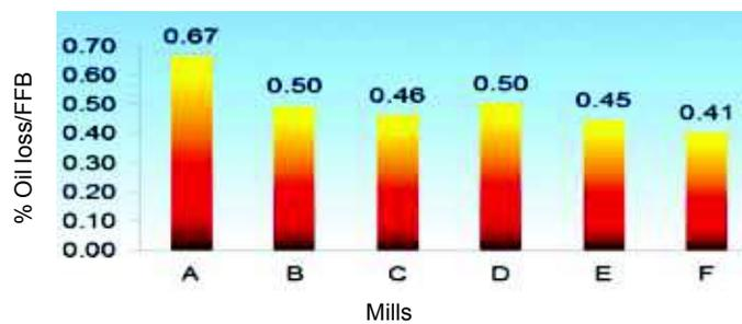
Figure 10. Percentage of oil loss to fresh fruit bunches (FFB) from sludge from separator.
