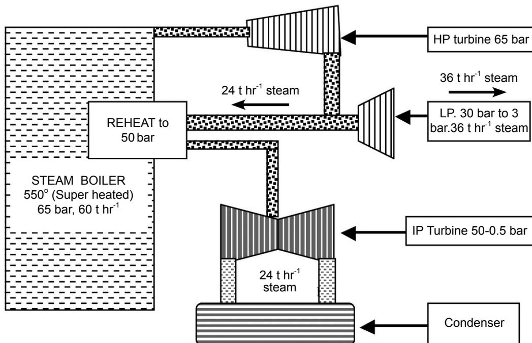
Figure 1. An example of a power plant cum process heating configuration.
