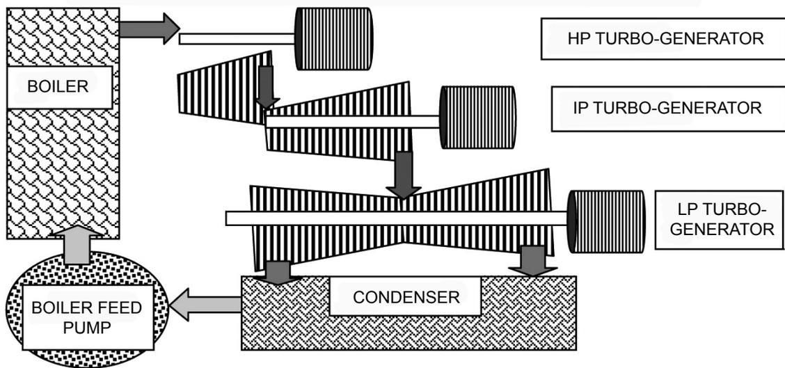
Figure 2. Schematic diagram of the supercritical pressure power plant.
