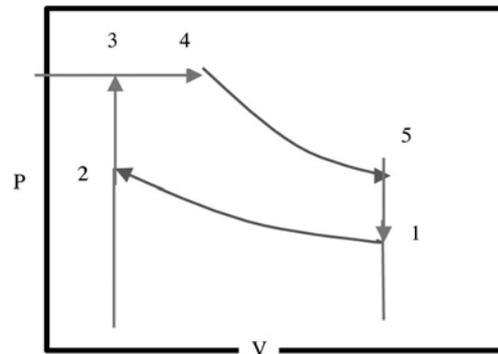
Figure 2. Dual combustion cycle (replaced diesel cycle).
