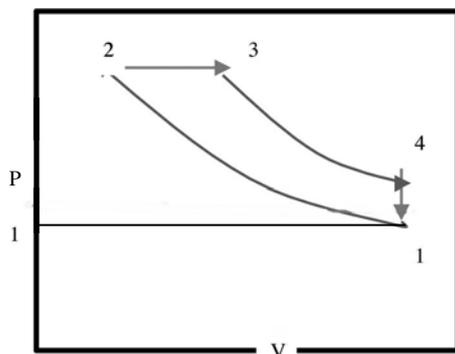
Figure 1. Diesel cycle (1892).
