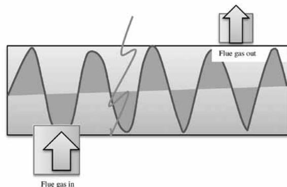
Figure 1. Heat transfer in shaft-less screw conveyor via counter flow direct contact with flue gas. Conveyor length: 20 m, conveyor diameter: 50 mm.
