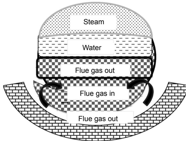
Figure 3. The flue gas path.
