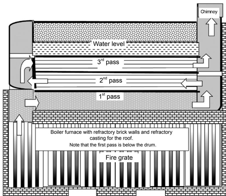
Figure 2. Stork three-pass fire tube boiler.
