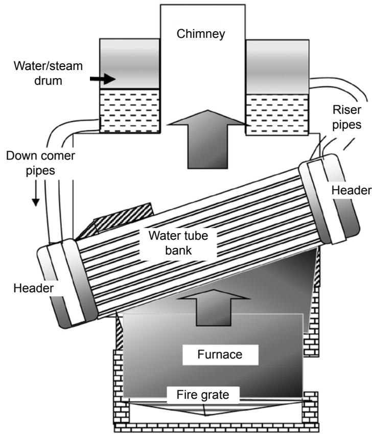
Figure 4. A vertical frazer water tube boiler.
