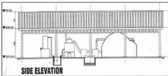
Figure 3. The layout of the taki carbonisation system (side elevation).
