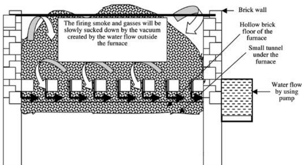
*Figure 1. Illustration of the hollow plinth brick carbonisation system.*
