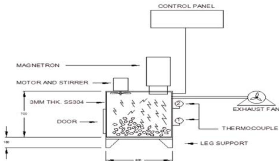
Figure 7. Schematic diagram of microwave carbonisation system.
