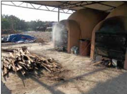
Figure 4. The carbonisation process, using the used wood as fuel.
