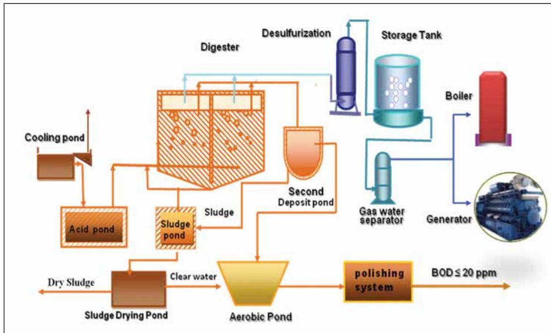
Figure 2. Biogas system for POME.
