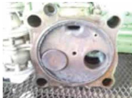
Figure 3. Condition of the combustion chamber of a gas generator using biogas for > 10 000 hr.
