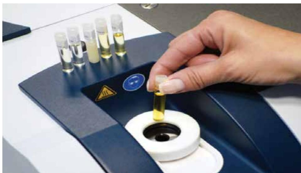
Figure 1. Rapid oil analysis with FT-NIR using disposable glass vials.
