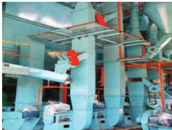
Figure 6. The four-stage dry separation for a cracked mixture.
