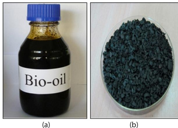
Figure 3. Pyrolysis products: (a) bio-oil and (b) bio-char.
