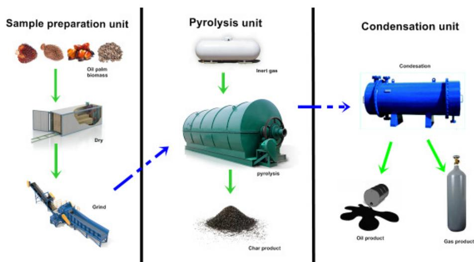
Figure 1. Reactor components in pyrolysis of oil palm biomass.
