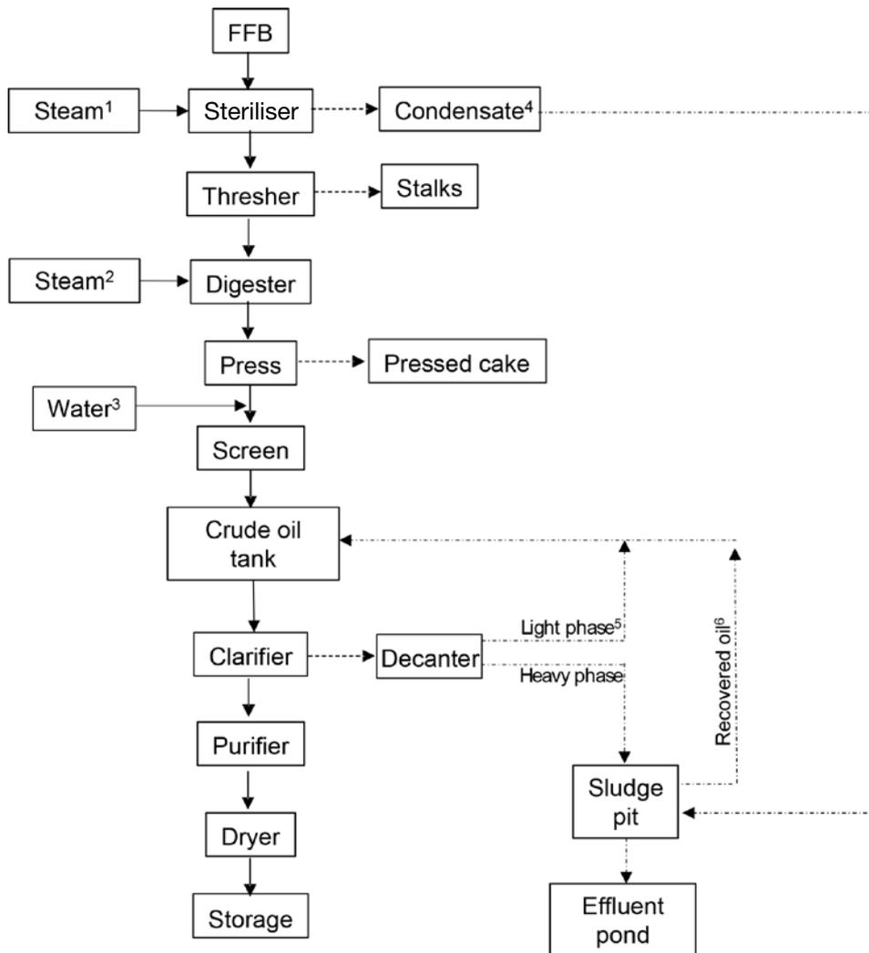
Figure 1. Flow chart for crude palm oil (CPO) extraction.
