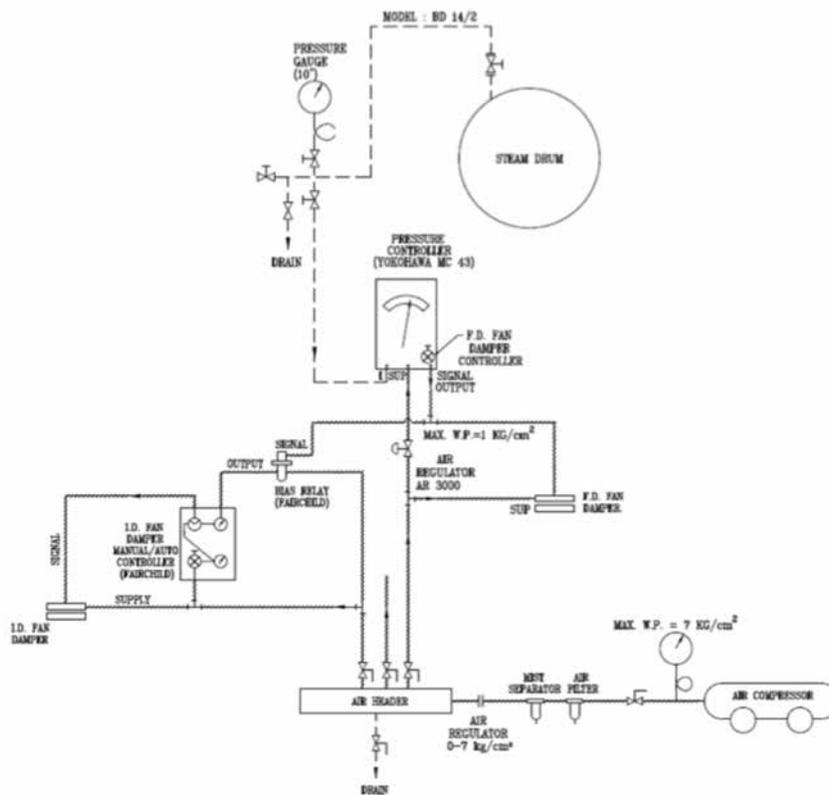
Figure 1. The conventional draught system comprising the ID and FD fans.
