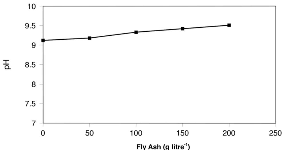
*Figure 1.* The pH of filtrates treated with various dosages of fly ash.
