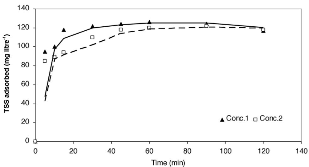
Figure 5. Adsorption of TSS by fly ash.
