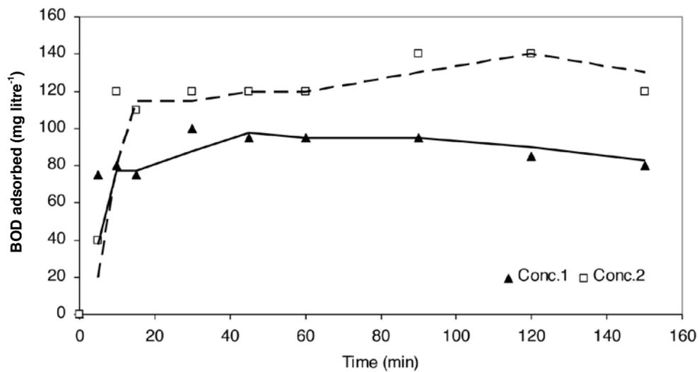
Figure 4. Adsorption of BOD by fly ash.
