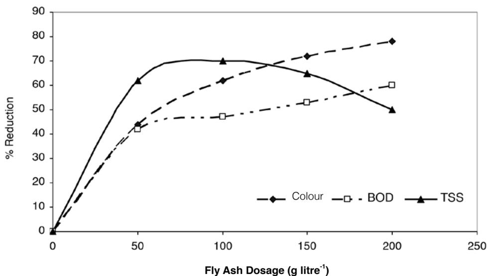
Figure 2. Impurities in filtrates treated with various fly ash dosages.
