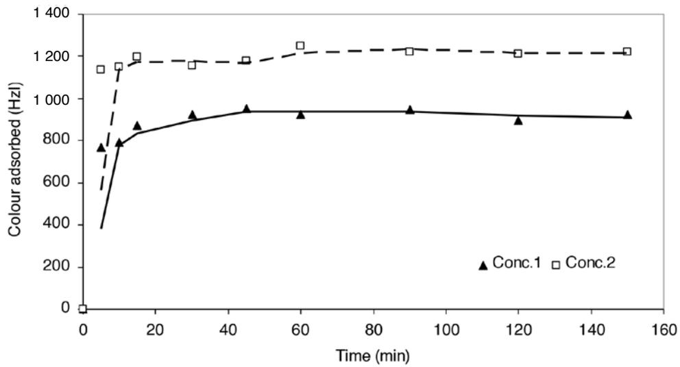
Figure 3. Adsorption of colour by fly ash.
