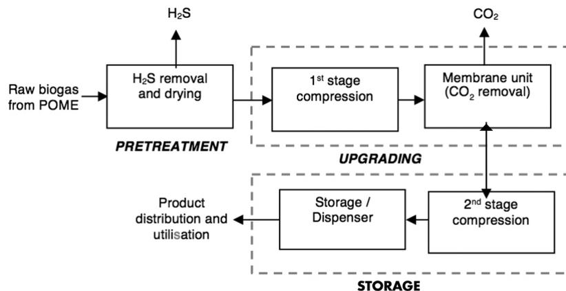
Figure 3. Process flow diagram for the production of bio-compressed natural gas (Bio-CNG) from palm oil mill effluent (POME).
