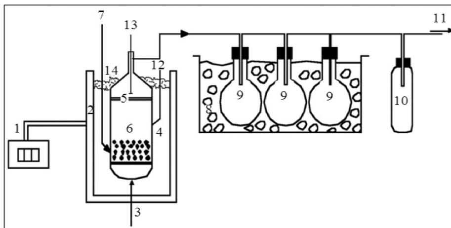
(1) Temperature recorder; (2) Furnace; (3) Fluidising gas; (4) Reactor; (5) Quartz frit; (6) Sand bed; (7) Feedstock inlet; (8) Water-ice bath; (9) Bio-oil collector; (10) Gas dryer; (11) Gas exit; (12) Sand feeder; (13) Thermocouple; (14) Glass wool.
