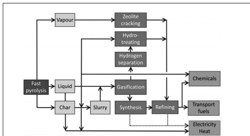
Figure 3. Bio-refinery concept for pyrolysis plant (Bridgwater, 2012).
