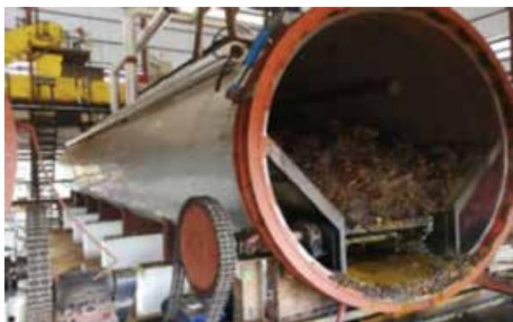
Figure 3. A horizontal steriliser with built-in conveyor.
