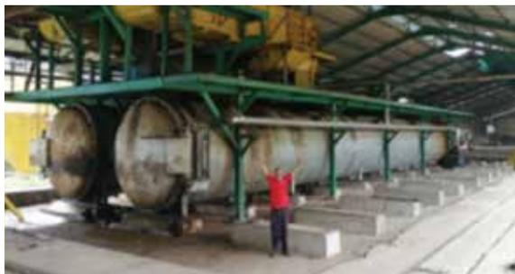
Figure 1. Static walking steriliser.
