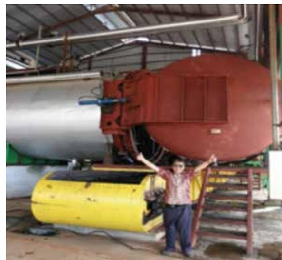
Figure 2. A single door for feeding fresh fruit bunch (FFB) into the steriliser.
