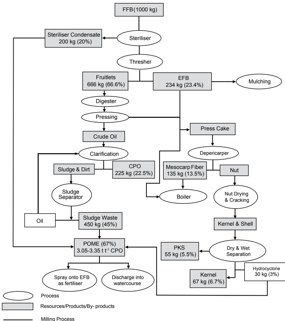
Figure 1. Brief description of palm oil milling process and current practices (Ma, 1999; Vijaya *et al.*, 2008; Liew *et al.*, 2015; Ropandi *et al.*, 2017).
