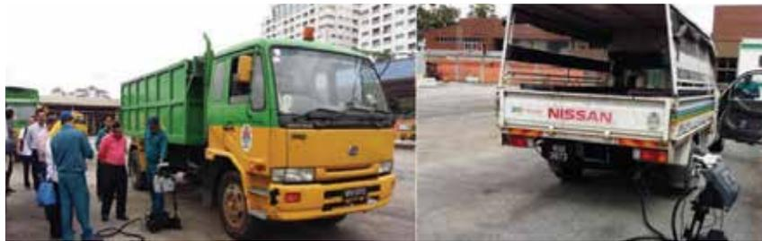
Figure 7. Smoke test by Department of Environment (DOE).
