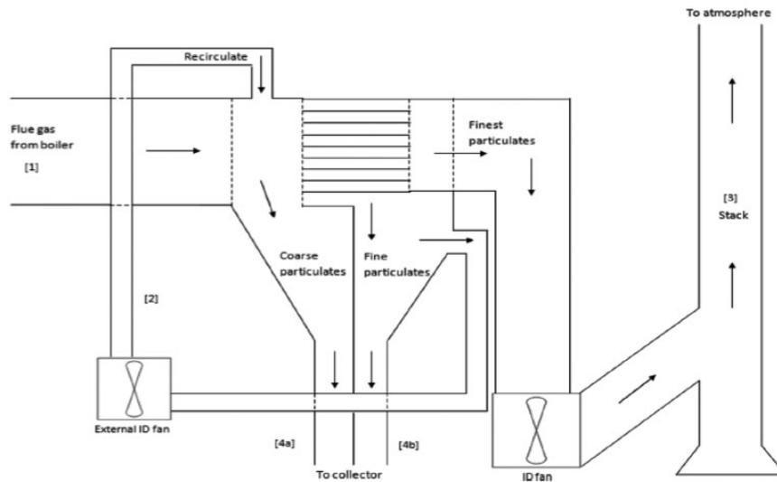
Figure 2. Modified multi-cyclones unit.
