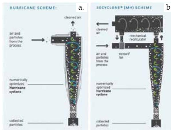
Figure 3. Cyclone-based technology; (a) Hurricane system and (b) ReCyclone.
