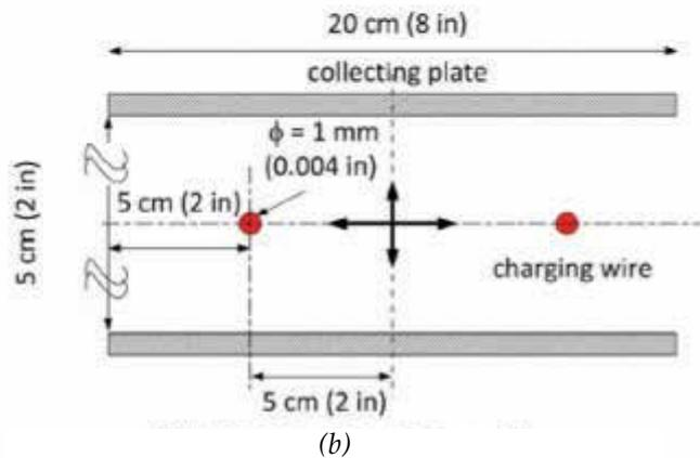
Figure 6. (a) Optimised wire-plate ESP design, and (b) ESP module.
