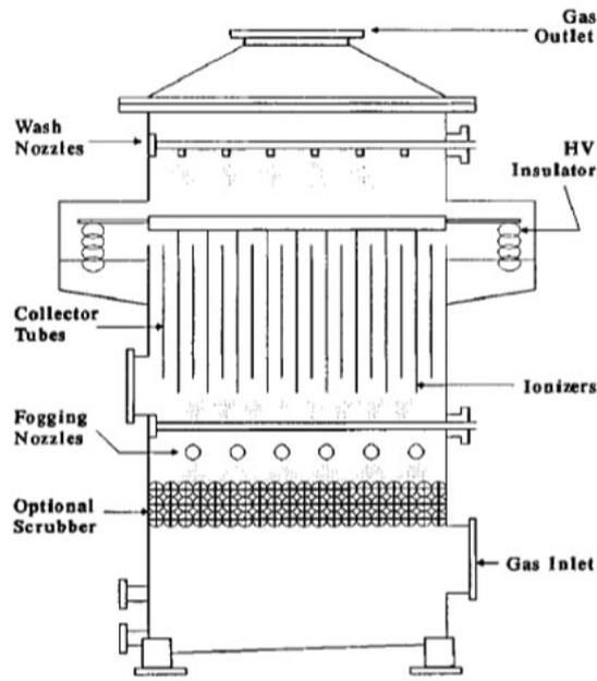
Figure 5. Schematic layout of wet tubular electrostatic precipitator.
