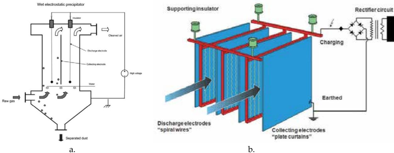
Figure 4. Electrostatic precipitator; (a) Wet ESP and (b) Dry ESP.
