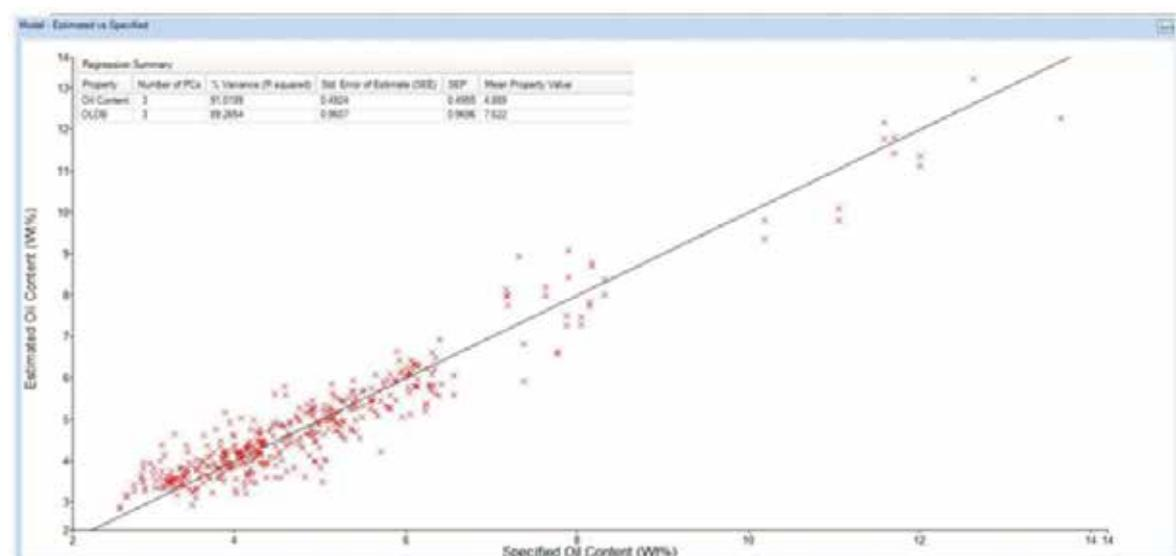
Figure 1. Oil content calibration model based on specific oil content (from wet chemistry analysis) and estimated oil content (modelled via chemometric algorithm).
