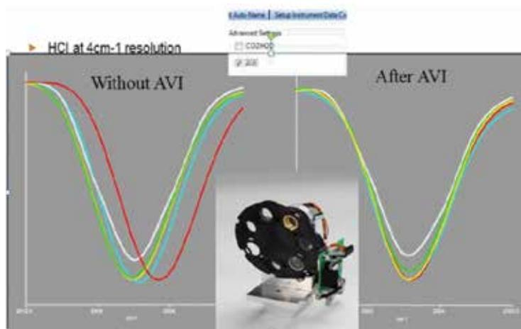
Figure 3. HCl peaks from different FTIR instruments with and without the AVI correction.
