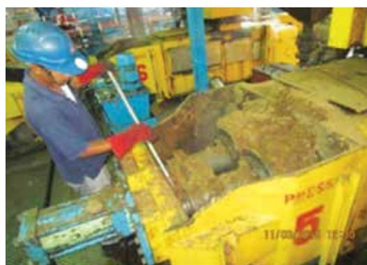
*Figure 4. The screw presses are used to extract oil after digestion process.*
