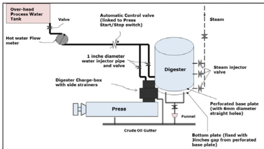
Figure 3. Hot water injection into digester.
