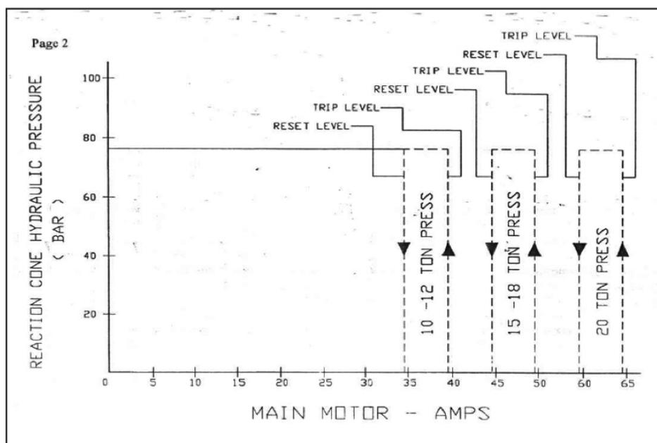
*Figure 5. The recommended cone pressure and motor load setting for three types of screw presses.*
