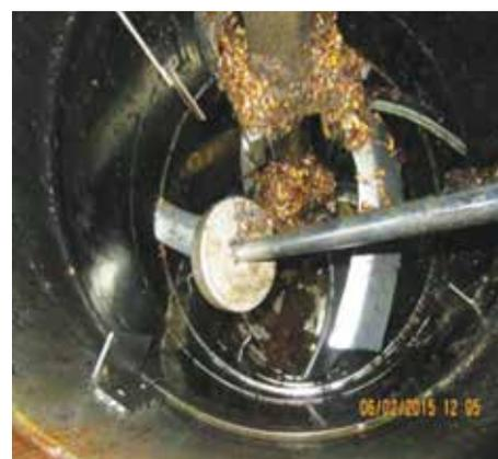
*Figure 2. The digester is used to mash the sterilised fruits.*
