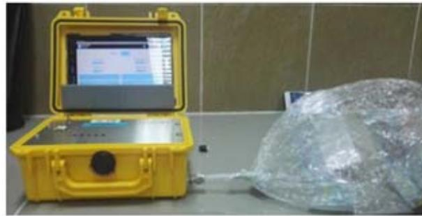
Figure 6. OdoTracker TR8 portable gas sensors for  $\text{H}_2\text{S}$  and  $\text{NH}_3$  level determination.
