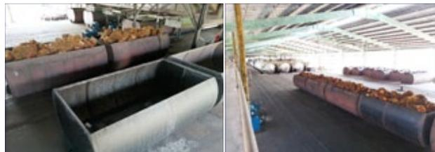
Figure 1. Fresh fruit bunches (FFB) are loaded into rusty cages in open holding area.
