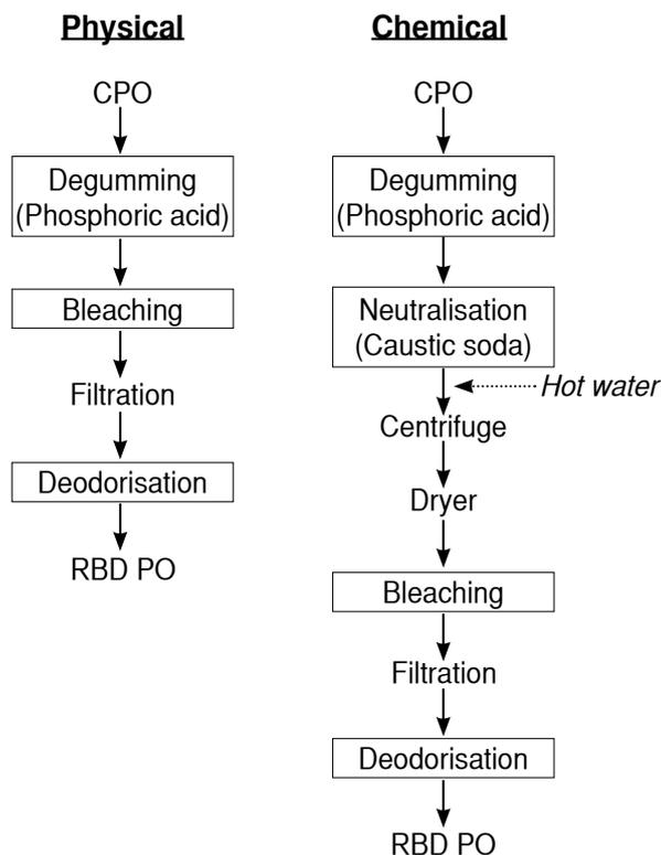
Figure 4. Flowchart of physical and chemical refining.
