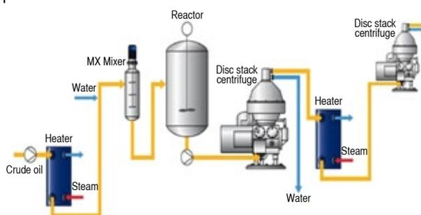
*Figure 3. Typical crude palm oil (CPO) washing process flow.*
