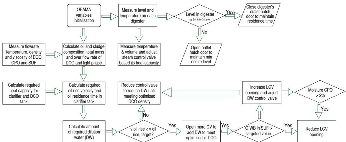
Figure 4. Flow Chart of the OBAMA-6 Control Algorithms.
