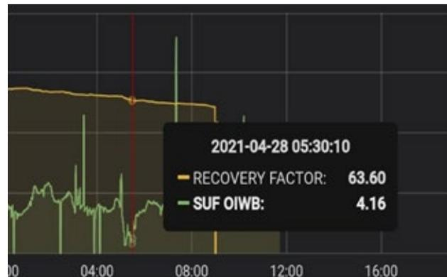
Figure 16. Reduction in OIWB% in SUF is possible down to less than 5%.
