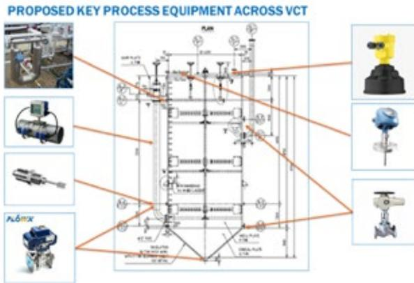
Figure 9. Typical equipment installed within a clarifier tank.
