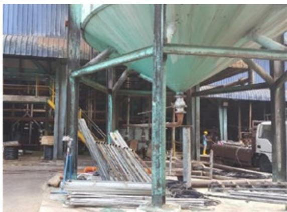
Figure 24. Position of discharge control valve to evacuate sludge at the bottom conical.
