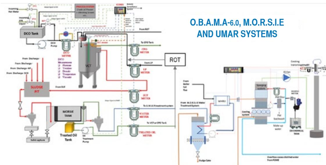
Figure 3. Integrated operations in reducing oil loss, foul odour, black emission and clean water recycling.
