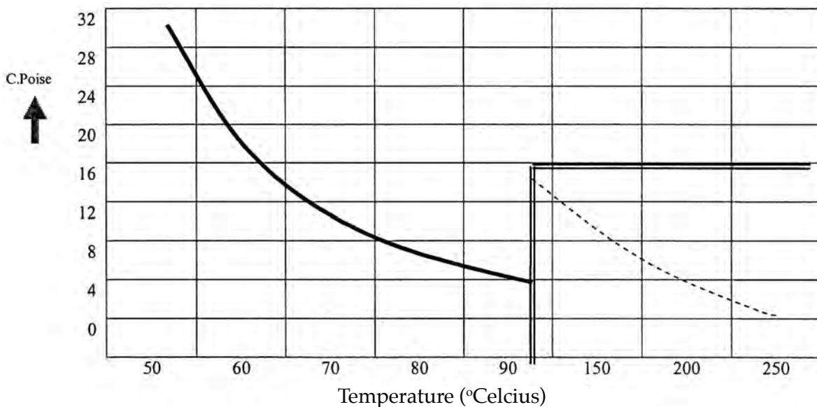
Figure 1. Effect of crude oil temperature on viscosity.
