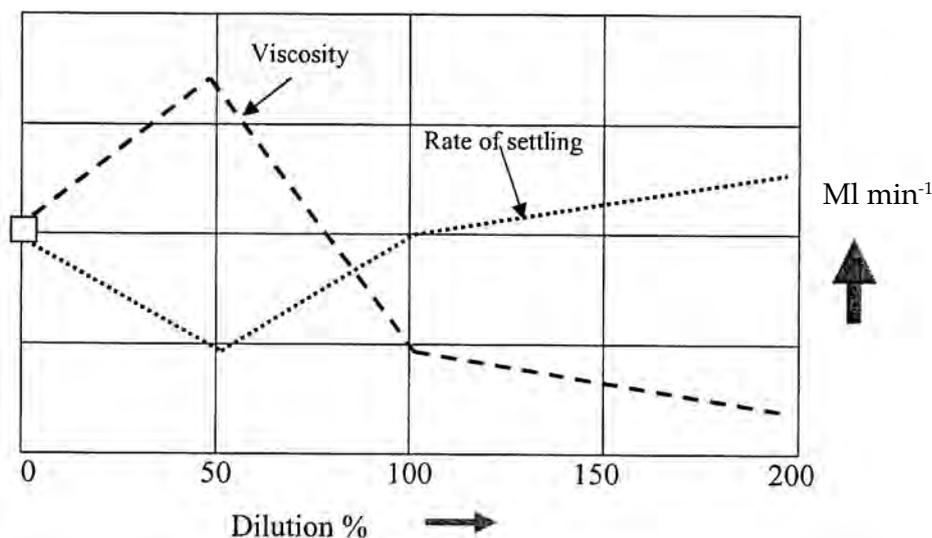
Figure 2. Dilution rate and rate of separation of crude oil.
