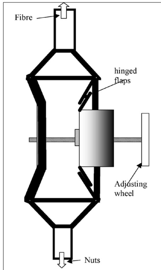
Figure 3. A simple method of adjustable flap construction.
