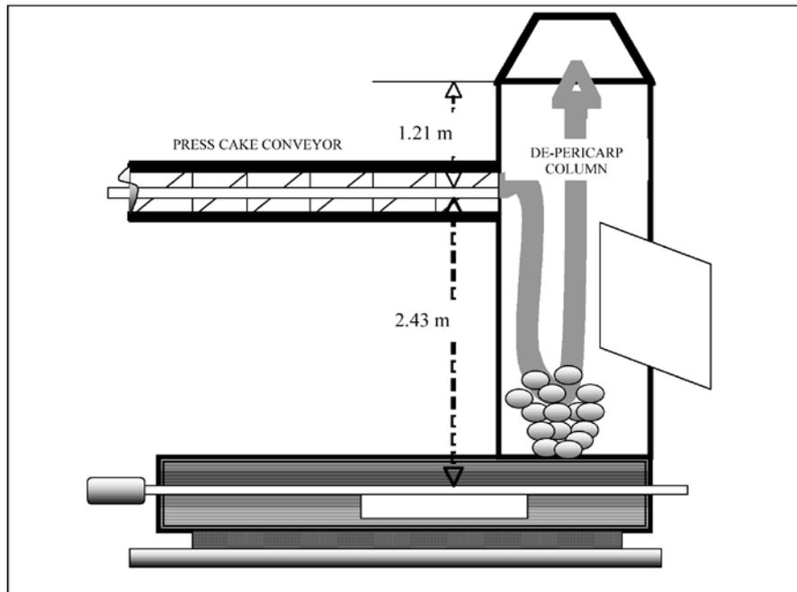
Figure 1. Dropping height of nut from the P.C conveyor.
