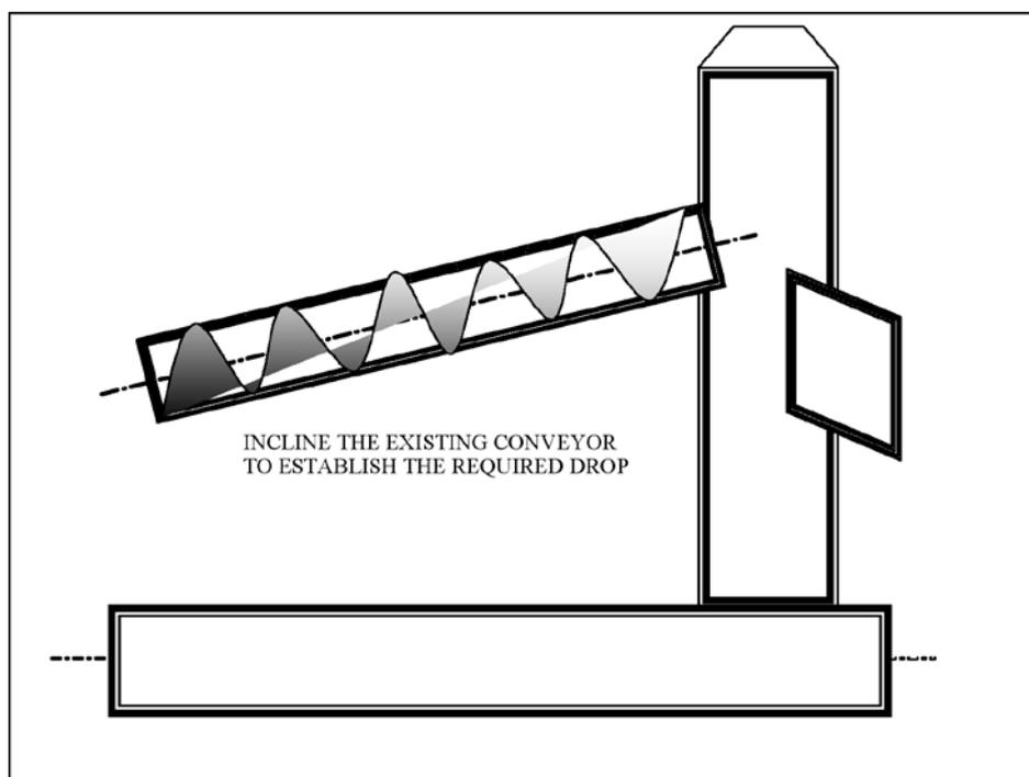
*Figure 2. Solving the problem by inclining the existing conveyor.*
