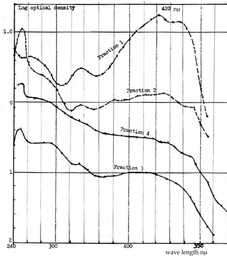
Figure 3. Absorption spectrum of fraction of palm oil of 24.7 peroxide value obtained by chromatography on Brockmann alumina using petroleum ether as eluting medium.
